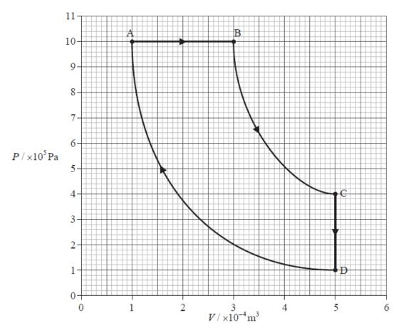
In the changes of state B to C and D to A, the gas behaves as an ideal gas and the changes in state are adiabatic.
