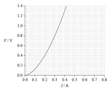
The variable resistor in the circuit in (c) is replaced by this non-ohmic conductor.
